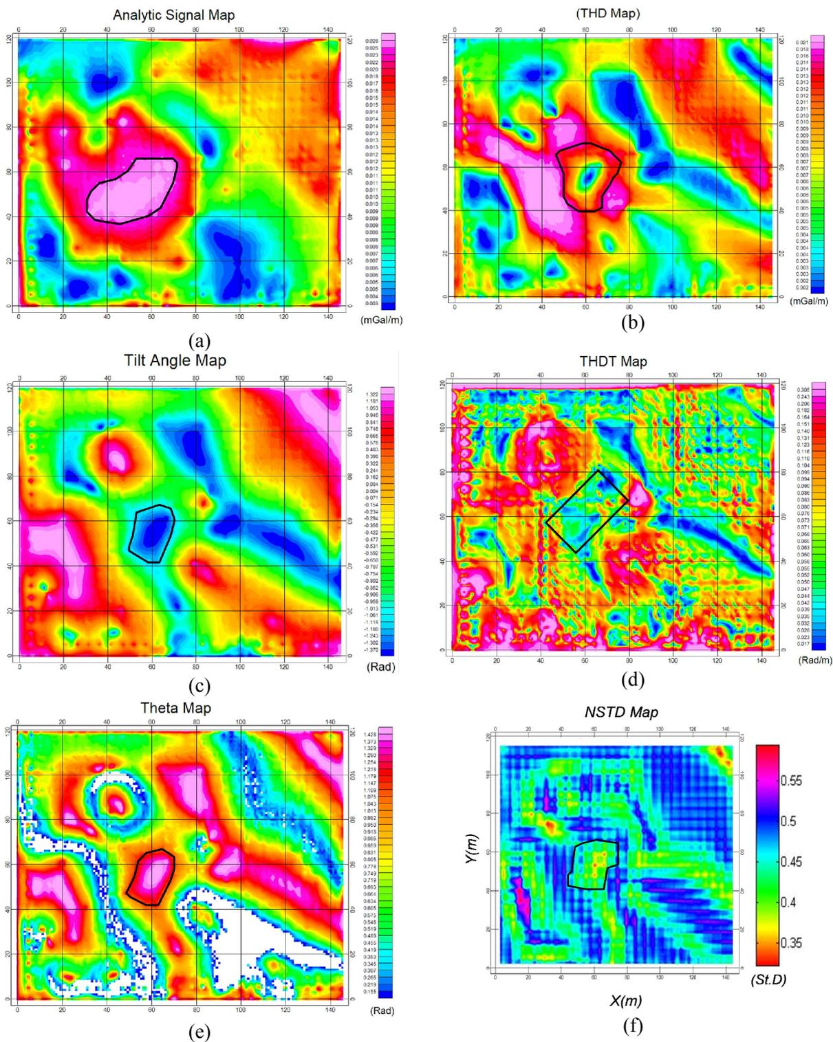
**Figure 6.** Results of applying edge detection methods to gravity anomalies of Dehloran Bitumen, (a) Analytic Signal, (b) THD, (c) Tilt Angle, (d) THDT, (e) Theta map, (f) NSTD.
