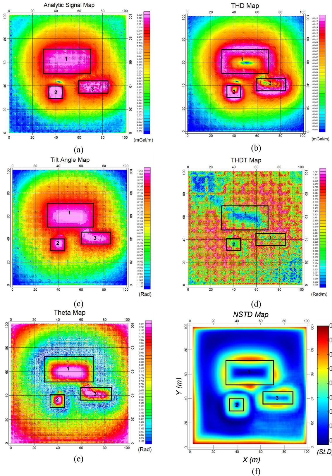
Figure 3. Results of applying edge detection methods to gravity anomalies of synthetic models, (a) Analytic Signal, (b) THD, (c) Tilt Angle, (d) THDT, (e) Theta map, (f) NSTD.
