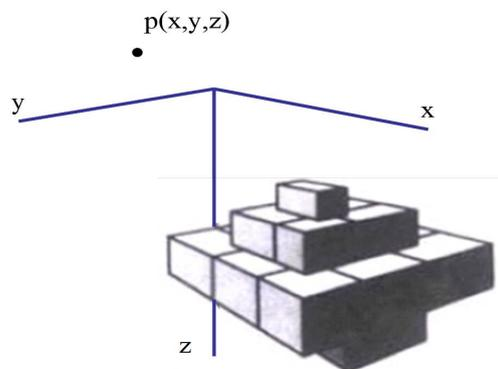
**Figure 1.** Approximation of the 3D mass by a collection of rectangular prisms to simulate different bodies (Blakely, 1995).
