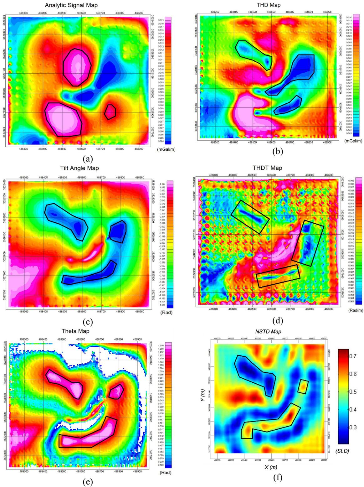
Figure 9. Results of applying edge detection methods to gravity anomalies of karst zones in SabzKoh, (a) Analytic Signal, (b) THD, (c) Tilt Angle, (d) THDT, (e) Theta, (f) NSTD.
