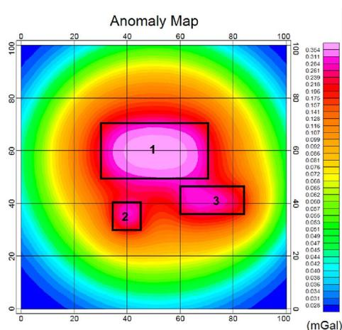
**Figure 2.** Gravity anomaly of synthetic models assuming properties shown in Table 1.
