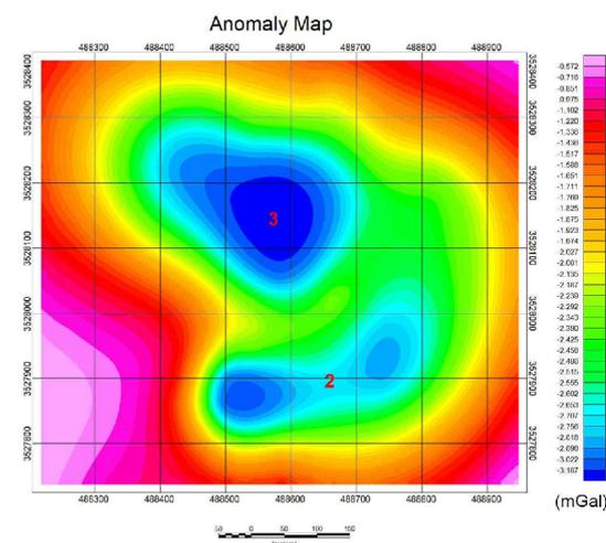
Figure 8. Residual gravity anomaly for zones 2 and 3 Shown in Figure 7.
