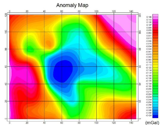
Figure 5. Residual gravity anomaly of Dehloran bitumen.
