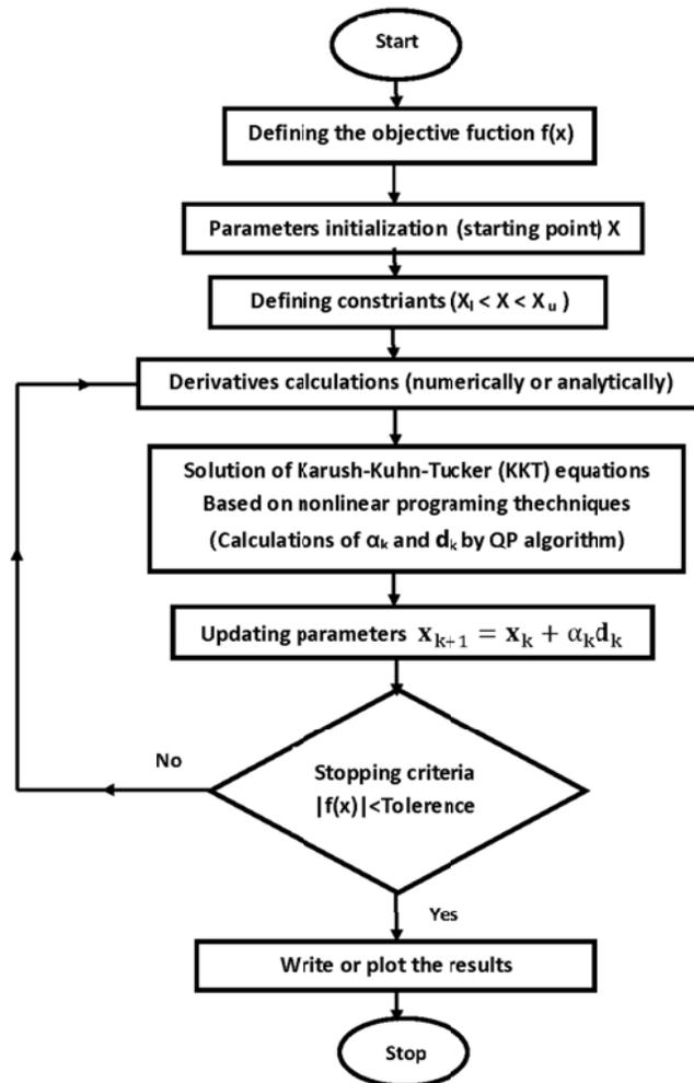
Figure 1. Flowchart of the non-linear constrained optimization algorithm.
