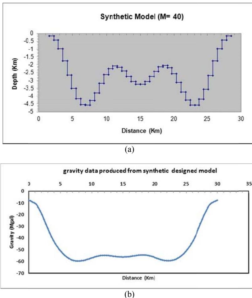
**Figure 2.** Designed synthetic model composed of 40 elementary prisms whose bottoms make interface between basement and sediments (a). Gravity response of the synthetic model (b).
