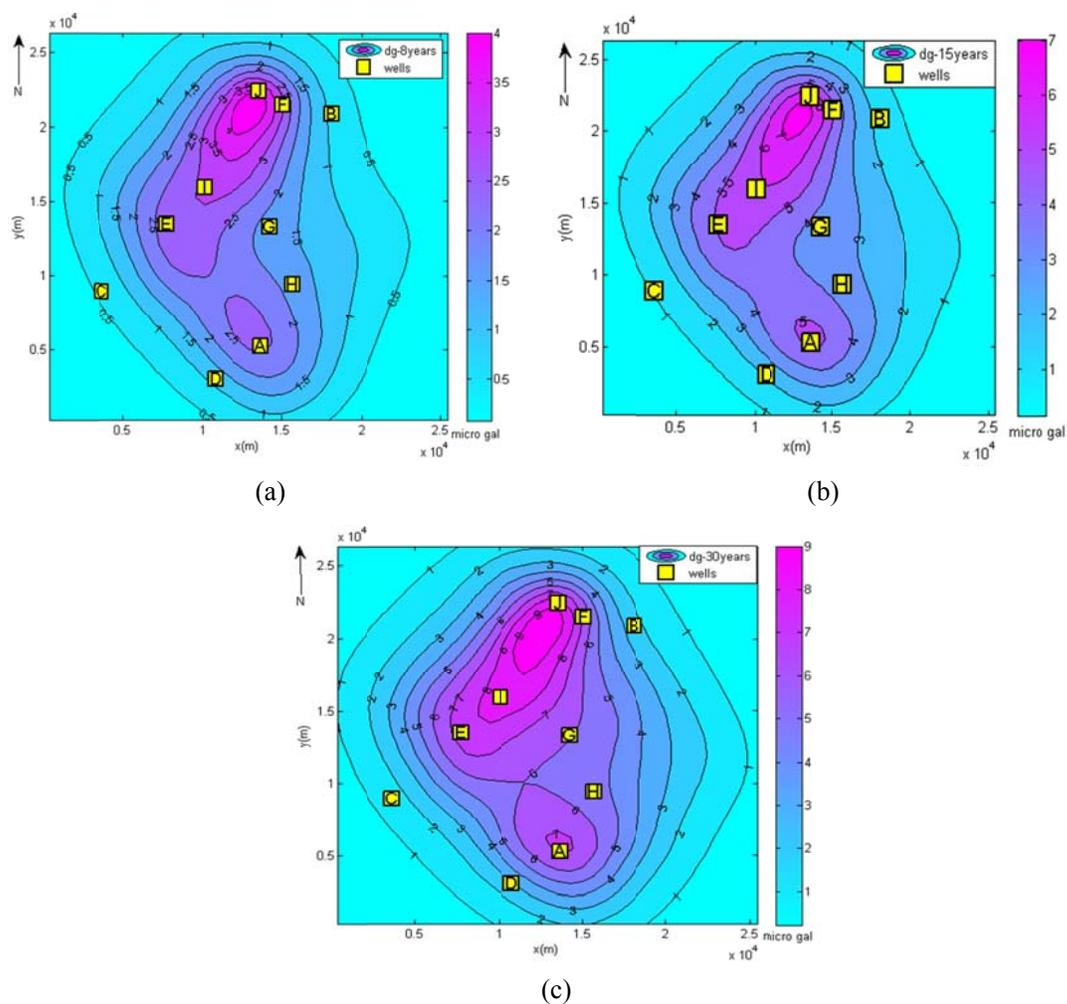
**Figure 3.** The results of achieved gravity signal for the scenario of reservoir depth 3500 m and 10 production wells. Figures 3a, 3b, and 3c show the gravity changes due to saturation variations in time intervals of 8, 15 and 30 years of production respectively.
