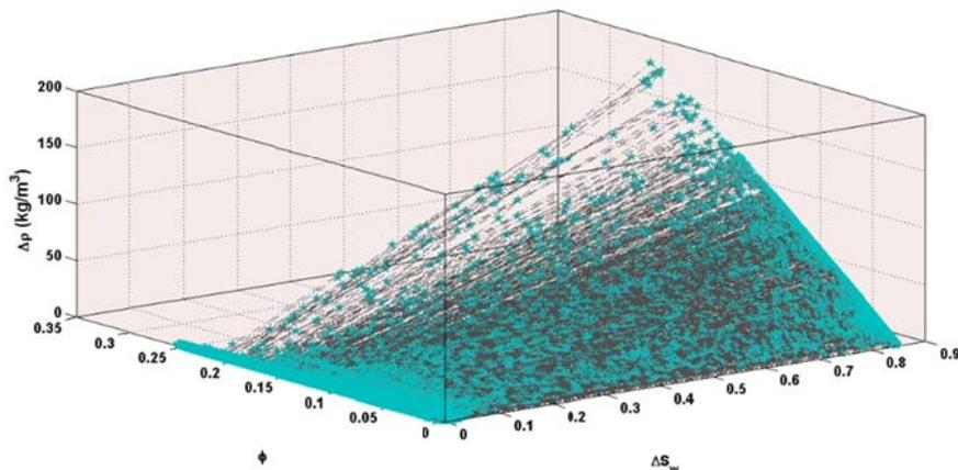
**Figure 2.** The scheme of relationship between water saturation changes ( $\Delta S_w$ ) and density changes ( $\Delta\rho$ ) after 30 years of production (2000-2030) with porosity ( $\phi$ ) throughout the reservoir.
