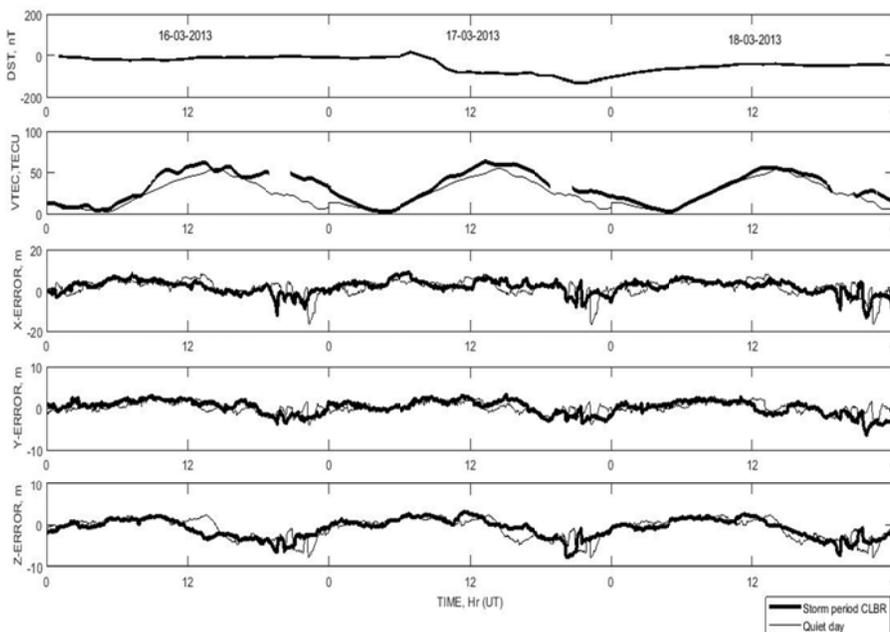
Figure 4. CLBR– Coordinates error with TEC during March 17, 2013 storm.
