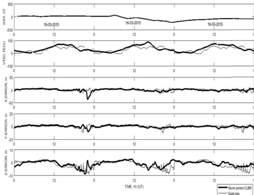
Figure 3. CLBR – Coordinates error with TEC during March 17, 2015 storm.
