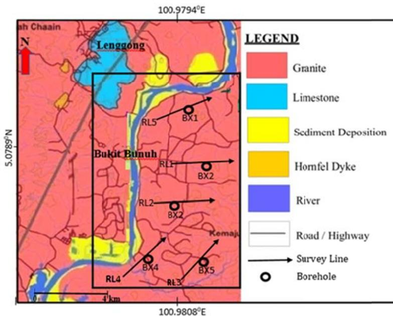
**Figure 1.** Geology map of Lenggong Valley with study area marked in the black box showing arrangement of resistivity survey lines and borehole locations (modified after Hidayah, 2015).
