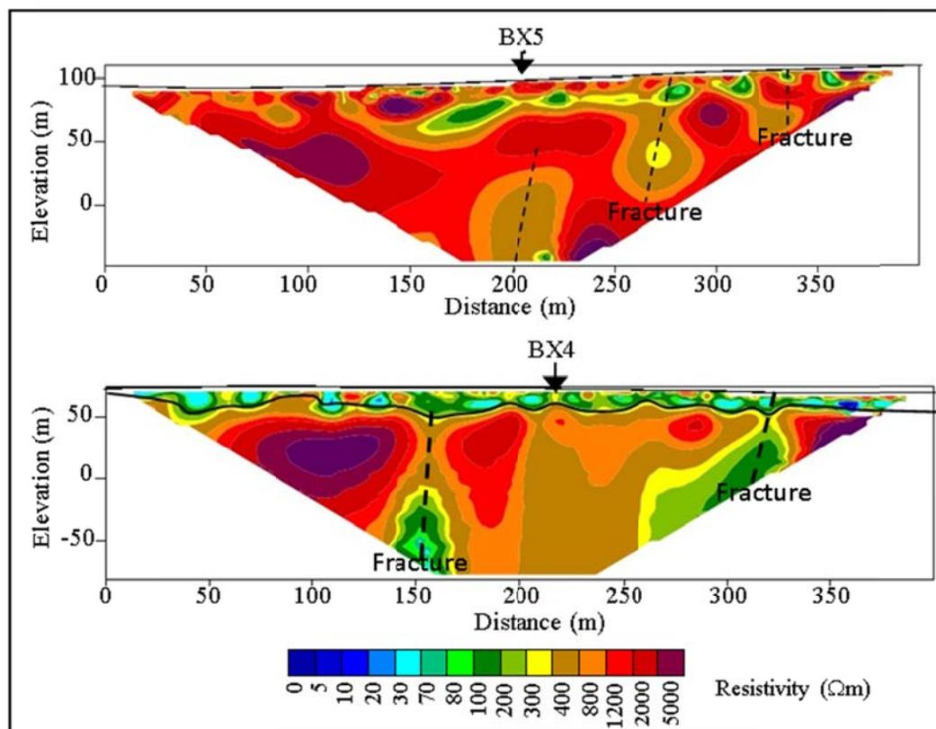
Figure 4. 2-D resistivity model of (a) RL3 and BX5 and (b) RL4 and BX4.
