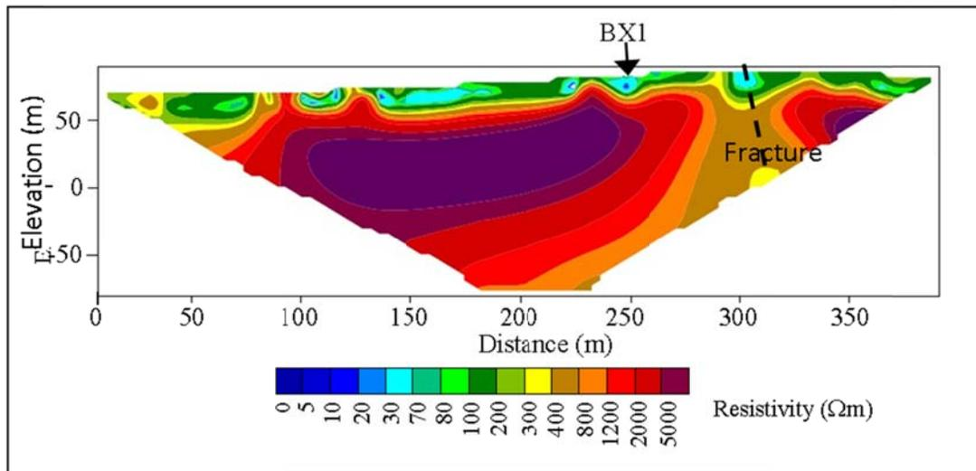
Figure 5. 2-D resistivity model of RL5 and BX1.
