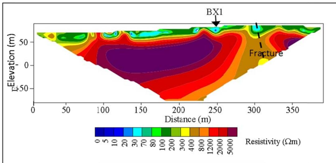
Figure 5. 2-D resistivity model of RL5 and BX1.
