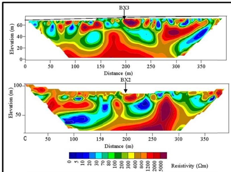
Figure 3. 2-D resistivity model of (a) RL1 and BX3 and (b) RL2 and BX2.
