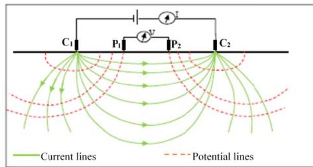
**Figure 2.** Four-point electrode configuration showing current and potential distribution (Modified from Nordiana et al., 2012).
