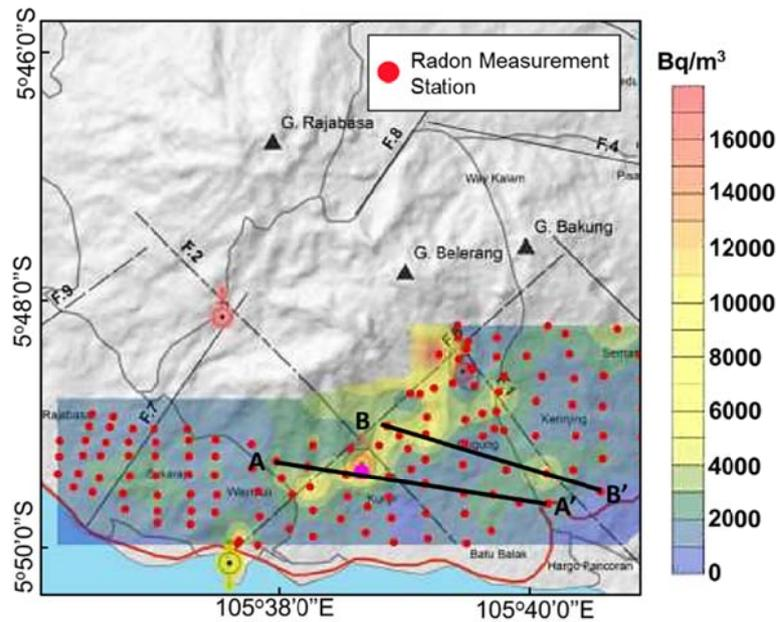
Figure 15. Radon measurement map in Rajabasa Geothermal field.
