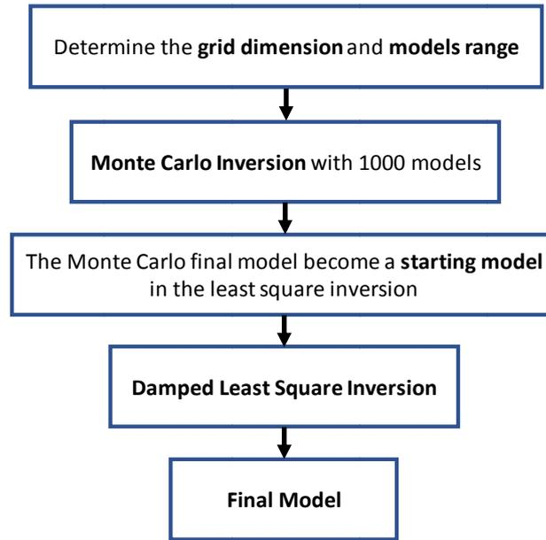
**Figure 9.** The purposed inversion scheme flow chart.
