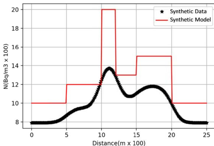
Figure 4. Radon synthetic data at a depth of 70 cm under the surface with a measurement length of 2500 m.
