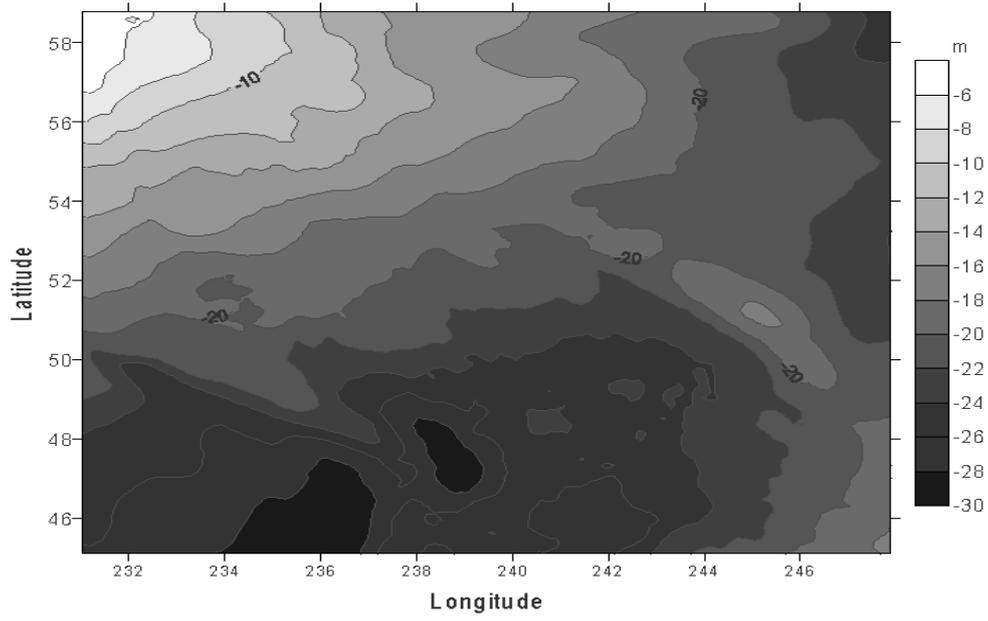
Figure 1. Geoidal heights through the direct numerical solution equations 10 and 14 (in meters).
