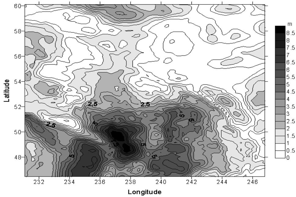
**Figure 3.** The differences between the geoidal heights computation through the direct numerical solution equations 10 and 14 and 1D FFT equations 11 and 14 (in meters).
