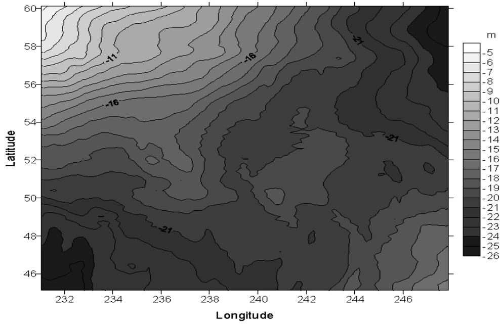
Figure 2. Geoidal heights through 1D FFT equations 11 and 14 (in meters).
