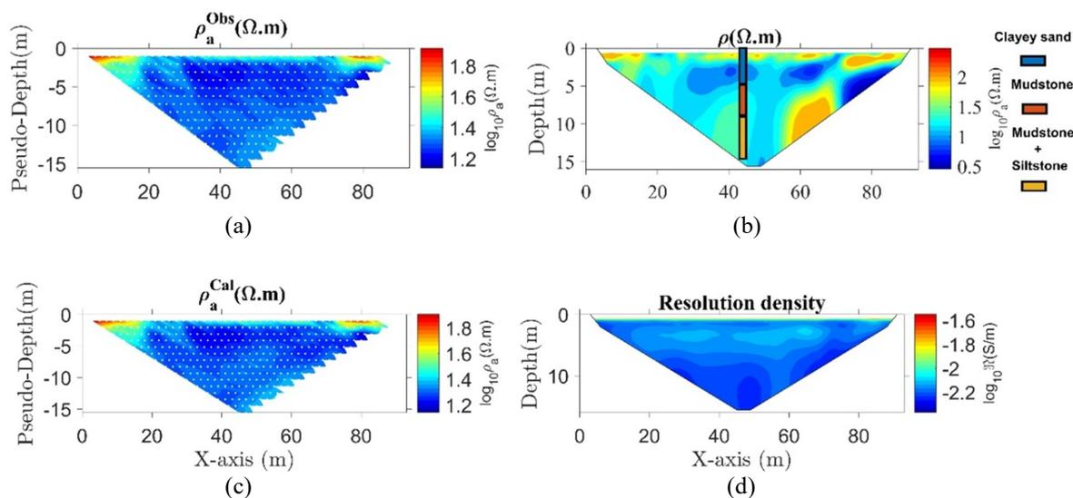
**Figure 4.** Inversion results of the field data without incorporating the reference model; a) The field data in a pseudo-section form, b) Inverted tomogram of the field data, c) The theoretical data set in a pseudo-section form, d) Resolution density  $\mathfrak{R}$  distribution corresponding to the inverted model. The water table measured in the borehole can be found in depth of about 3 m from the subsurface.
