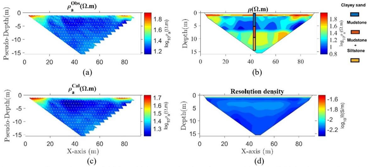
**Figure 5.** Inversion results of the field data with incorporating the reference model; a) The field data in a pseudo-section form, b) Inverted tomogram of the field data without incorporating the reference model, c) The theoretical data set in a pseudo-section form, d) Resolution density  $\mathfrak{R}$  distribution corresponding to the inverted model. The water table measured in the borehole can be found in depth of about 1.5 m from the subsurface.
