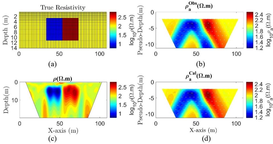
**Figure 1.** The resulting inversion of the first synthetic example; a) The true resistivity model including two rectangular bodies, one conductive (10  $\Omega m$ ) and the other resistive (1000  $\Omega m$ ), in a homogeneous medium of 100  $\Omega m$ , b) The noise-contaminated synthetic data set in a pseudo-section form, c) The inverted model based on the model-space Occam's inversion, d) The theoretical data set in a pseudo-section form.
