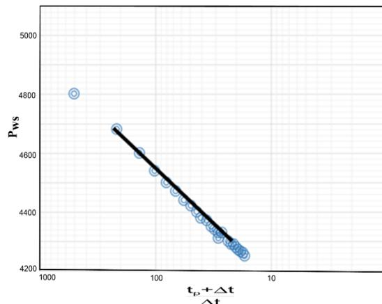
**Figure 3.** Interpretation of fall off test of B3 well.
