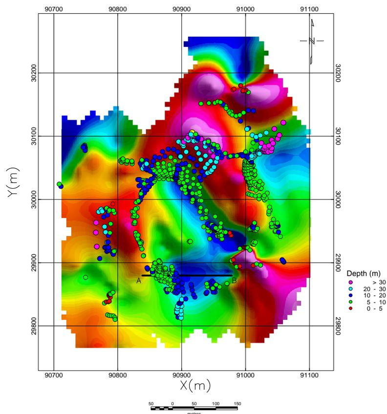
Figure 5. The Bouguer gravity anomalies (mGal) and Euler depths.
