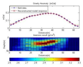
Figure 12. The density model obtained by inverting field gravity data (profile AA'). The subsurface is divided into  $26 \times 20 = 520$  cells of side 2.5 m. The density contrast and the geometry for manganese ore occurrence well recovered.
