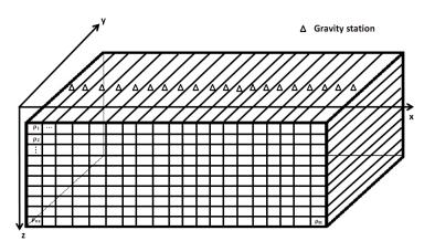
Figure 1. Discretization of the subsurface with infinity long horizontal prisms.
