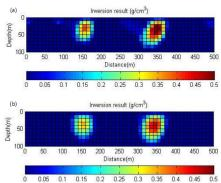
Figure 7. The density model obtained by inverting the gravity data of Figure 6 using minimum distance and smoothness constraints. Smoothness constraint is used in (a) with  $\zeta_{n_a} = \zeta_{n_a} = 0.01$  and (b) with  $\zeta_{n_a} = \zeta_{n_a} = 0.03$ .
