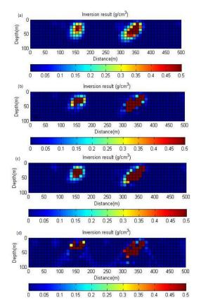
Figure 8. The density model obtained by inverting the gravity data of Figure 6 using minimum distance and compactness constraints for different values of  $\mathcal{E}$ . In (a), (b) and (d) the value of  $\mathcal{E}$  is  $10^{-1}$ ,  $10^{-2}$  and  $10^{-11}$ , respectively, while in (c)  $\mathcal{E}$  was chosen according to the trade-off curve method.
