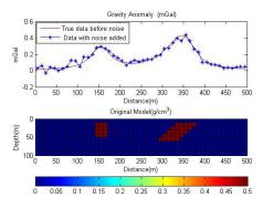
Figure 6. The synthetic model that used to test the inversion method. Contrast of densities for dipping and vertical dikes are  $0.5 g / cm^3$ . Gaussian noise with a zero mean and the standard deviation of 5% for the maximum datum is added.
