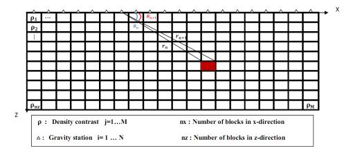
Figure 2. Cross-section of the model under gravity profile. Gravity stations are located at the center of the blocks at the ground surface. Cells are square and their dimensions are equal to the distance between two observation points.
