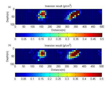
Figure 9. The density model obtained by inverting the gravity data of Figure 6 using minimum distance, smoothness and compactness constraints. The parameter  $\varepsilon$  is chosen according to the trade-off curve method and inversion is done for (a)  $\zeta_{H_t} = \zeta_{H_t} = 0.01$  and (b)  $\zeta_{H_t} = \zeta_{H_t} = 0.07$ .
