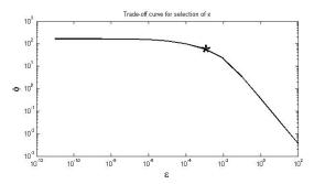
Figure 5. Trade-off curve that illustrates the selection of  $\varepsilon$  for the compactness constraint.
