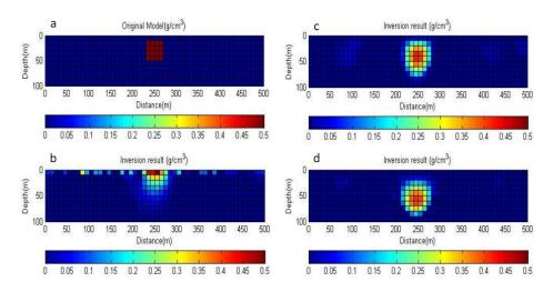
Figure 3. (a) Illustration of the effect of the depth weighting function. Original model is square with the dimensions of  $40 \times 40$  m. (b), (c) and (d) display inversion results for  $\beta = 0$ , 0.9 and 1.4, respectively.
