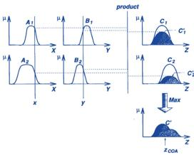
Figure 1. Graphic representation of Mamdani fuzzy inference method using multiplication and maximum operator (Jang et al., 1997).
