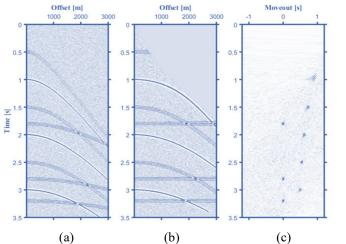
Figure 2. Synthetic data (a), NMO Gather (b) and Radon Transform of NMO gather (c).
