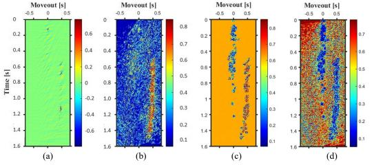
Figure 6. Initial radon transform (a), FIS output cluster including multiple energy (b), FIS output cluster including multiple and primary energy (c) and FIS output cluster including random noise (d). The color bar represents the magnitude of attributes.
