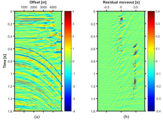
Figure 4. NMO Corrected Gather from Gulf of Mexico (a) and its parabolic radon transform (b). The color bar represents the amplitudes.
