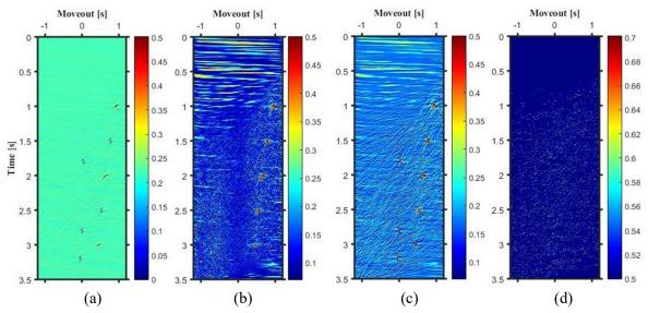
Figure 3. (a) Initial RT, (b) the class including the multiple parts, (c) the class including primary and multiple and (d) the class including random noise. The color bar presents the amplitudes.
